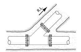
R.L. = RESTRAINED LENGTHS TO BE DETERMINED BY DESIGN ENGINEER
